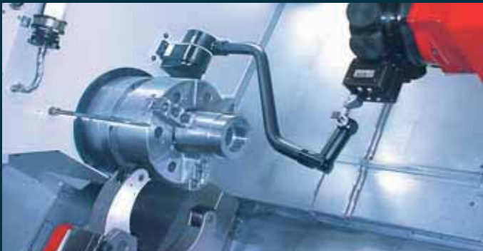
The automatic swivel measuring probe (optional) is used for tool measurement in the workspace.
