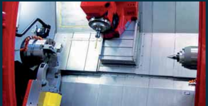
With the modular machine concept it is also possible to have a tailstock in combination with NC controlled steady-rest instead of the lower tool turret, depending on the customer's requirements. The steady-rest can be hydraulically lowered 250 mm as required.
