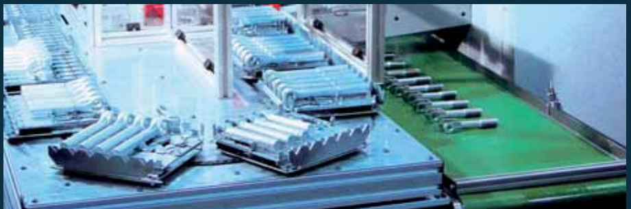
20-station pallet magazine with customer-specific pallets
