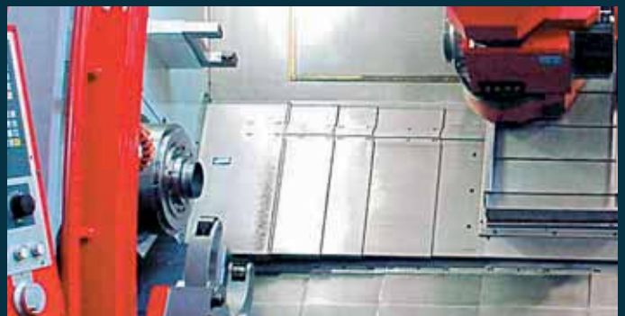
A laser measuring system (optional) can be installed to measure tools in the workspace on the machine variant with milling spindle.
