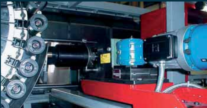
There is an integrated, safe, rocker-controlled tool changer for changing tools in the milling spindle. This picks up the tools from the 30/48/80-station magazine. This produces maximum flexibility.
