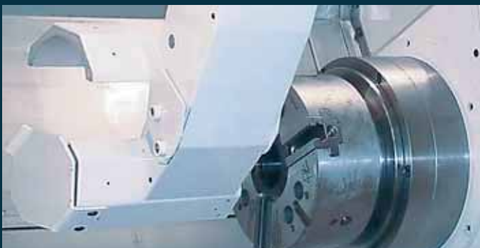
The HYPERTURN 690 can be fitted with a finished parts pick-up system (optional) for automatic removal of finished parts.
