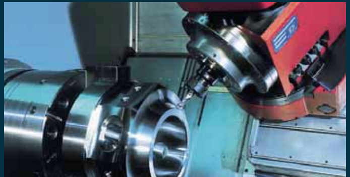
The upper turret is replaced by a 21 kW liquid-cooled milling spindle in the B axis version. The B axis travel range is 205°. This is infinitely variable with 0.001° resolution. In addition, the B axis can be clamped in any position with 5° indexing.
